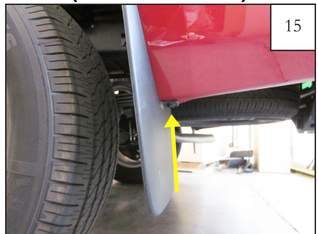
15 Remove one hex bolt from underside of mud flap using a 10mm socket. Discard mud flap.
