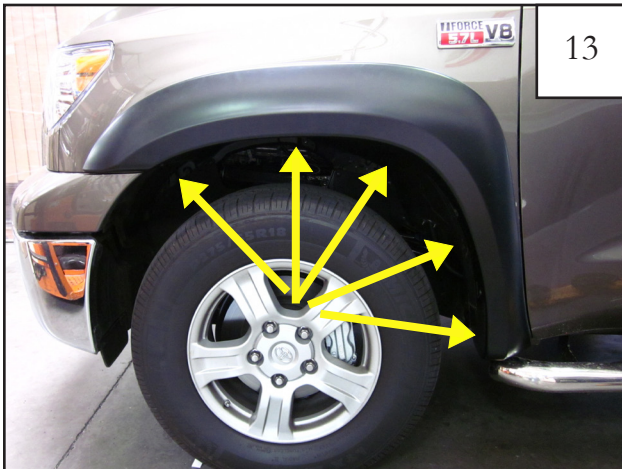
13 Ensure flare is properly positioned and tighten all screws.
