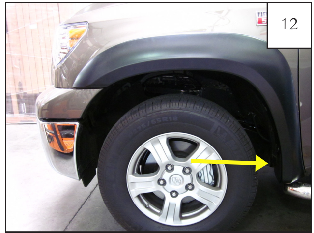
12 Screw (SW1-0036) lower rear wheel well location.
