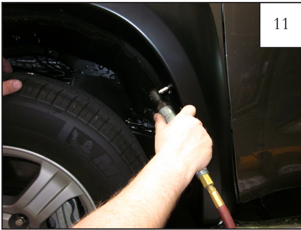
11 Start Screw (SW1-0036) through the one lower rear hole in flare and into factory hole in lower rear of wheel well.
