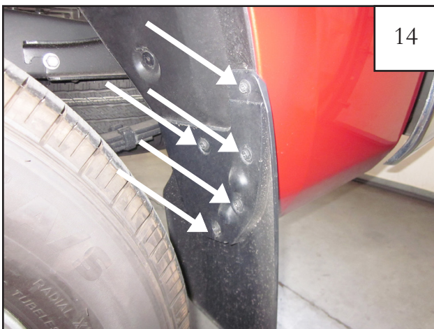
14 Remove five hex bolts from factory mud flap using a 10mm socket.
